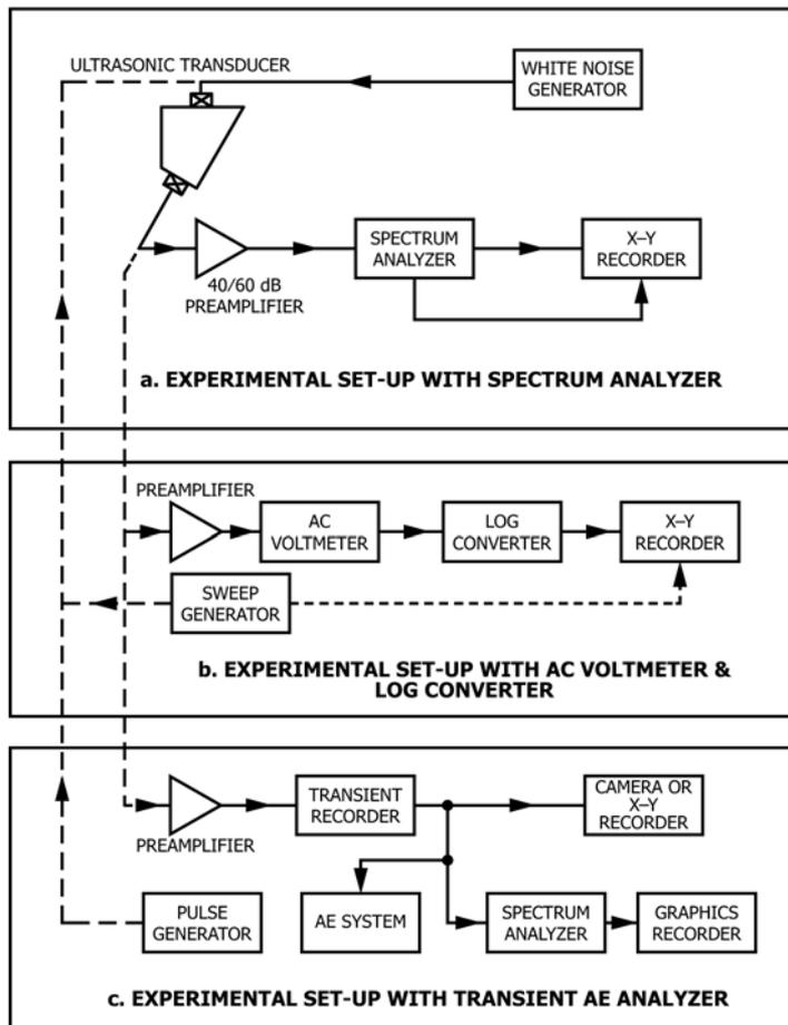
FIG. 1 Block Diagrams of Possible Experimental Setups
