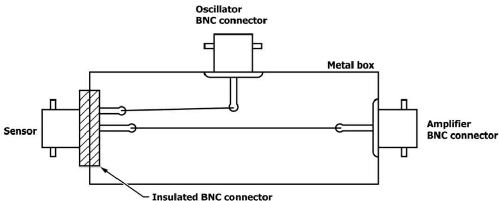
FIG. X2.1 Schematic of a Simple Voltage Insertion Box
