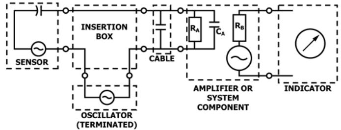
FIG. X2.2 Equivalent Circuit of the Voltage Insertion Measurement
