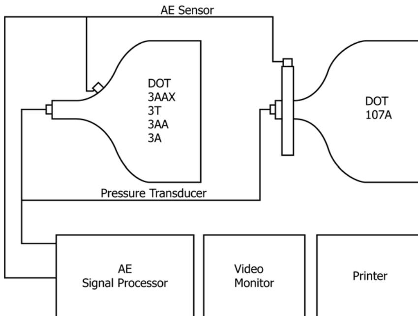
FIG. 1 Essential Features of the Apparatus with Typical Sensor Placements
