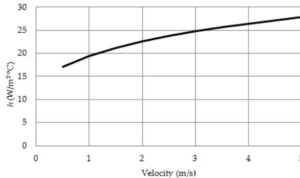
Figure D-4-2: Convective heat transfer coefficient ( $h$ ) as a function of velocity
