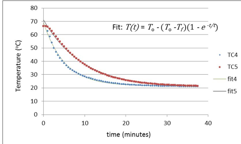
Figure B-2: Measured temperature vs. time together with calculated values using the thermal time constant,  $\tau$ , obtained from a least-squares-error fit to the experimental data
