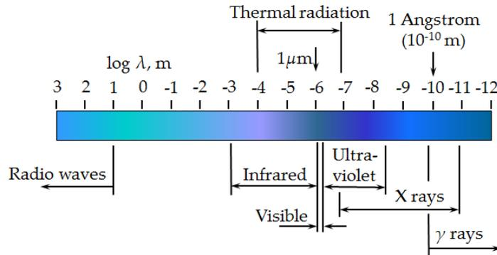
Figure D-6-1: Part of the Electromagnetic Spectrum
