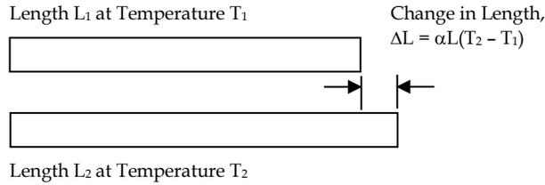
Figure 3.1-1: The Effect of Increase in Temperature on Length
