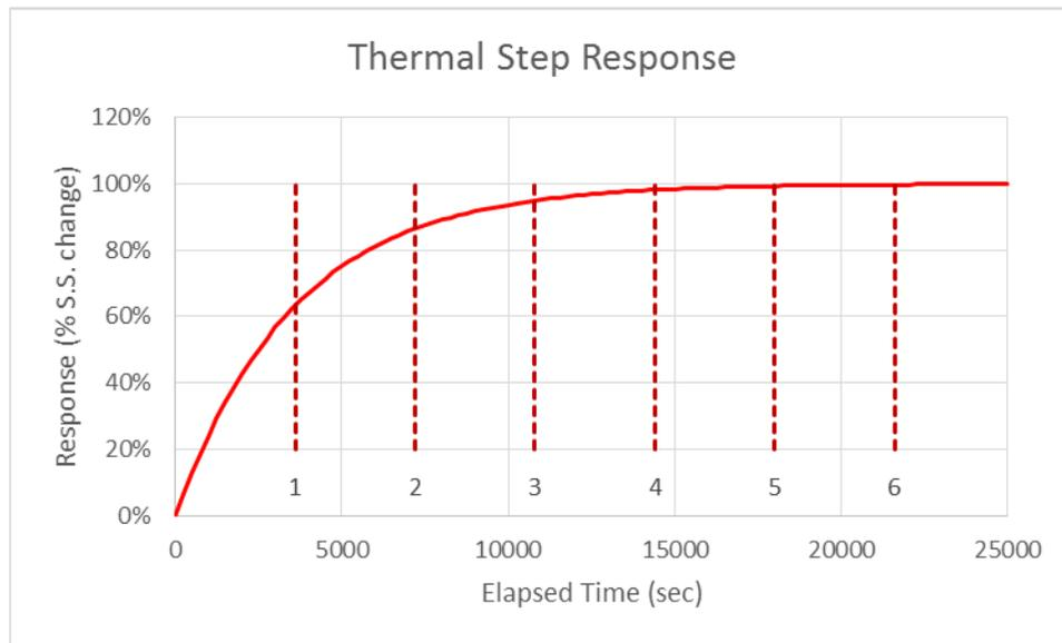
Figure 3.5.2-1: Thermal Step Response
