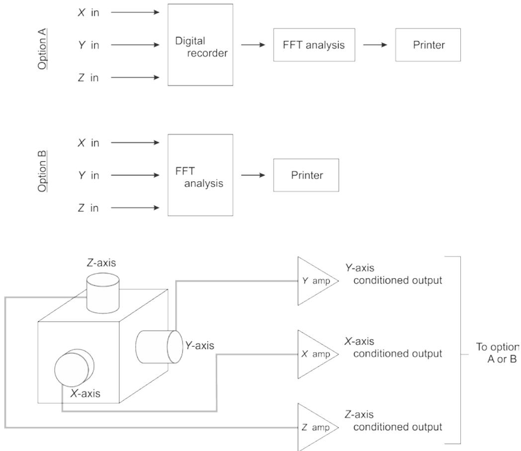
Figure G-8-1: Diagram of Sensor Arrangement and Instrumentation Configuration
