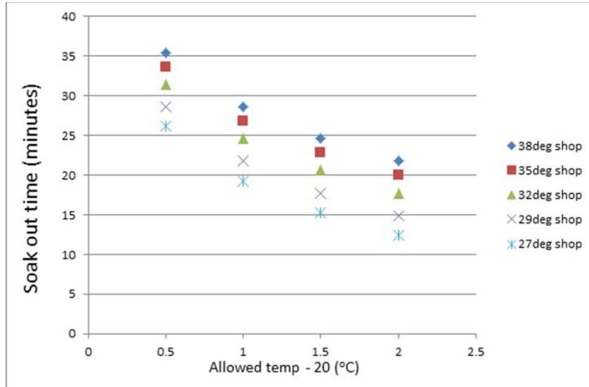
Figure B-3: Estimated soak out time for a workpiece coming from a shop area at some temperature into a CMM room with a nominal temperature of 20 °C
