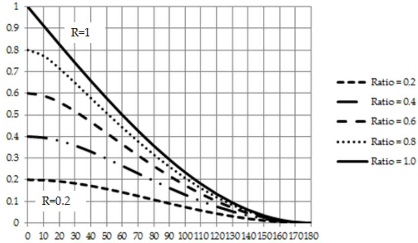
Figure D-3-3: Values of  $F_{1-2}$  for Assumed Values of the Ratio and Angle
