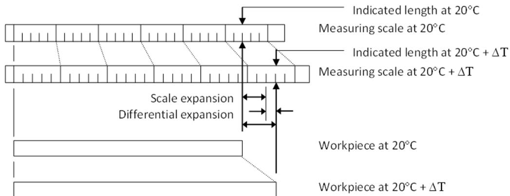
Figure 3.2-1 – The Effect of Differential Expansion on Length
