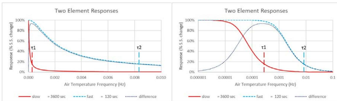
Figure 3.5.2-3: Differential Equation of Measuring System (a) Linear freq. Scale (b) Logarithmic freq. Scale
