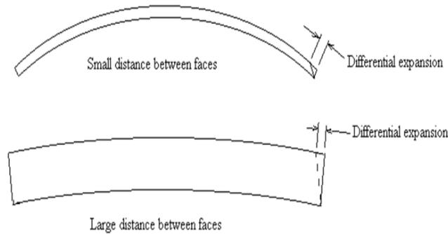
Figure F-2.3-1: Effect of Differential Expansion Relative to Distance between Beam Faces
