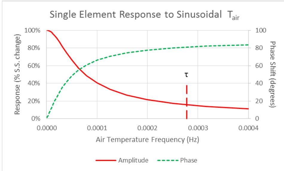
Figure 3.5.2-2: Thermal Response of a Simple Body to Temperature Variation
