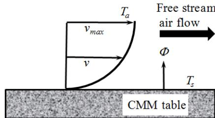
Figure D-4-1: Heat Transfer by Convection Showing Air Velocity Profile
