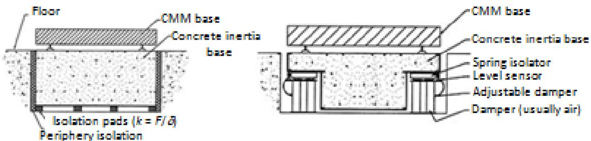
Figure 6.1-1: Passive and Active Isolation Systems
