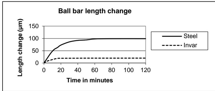
Figure B-1: Change in Ball Bar Length as a Function of Time
