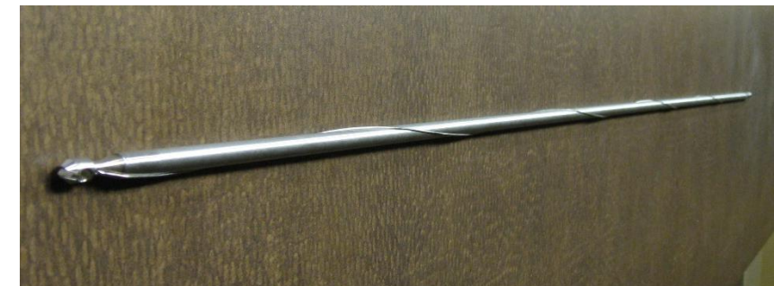
Mock-up of simulated wire-wrapped fuel pin
