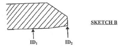
Reply (2):  $ID_2$  represents fitting weld bevel.
